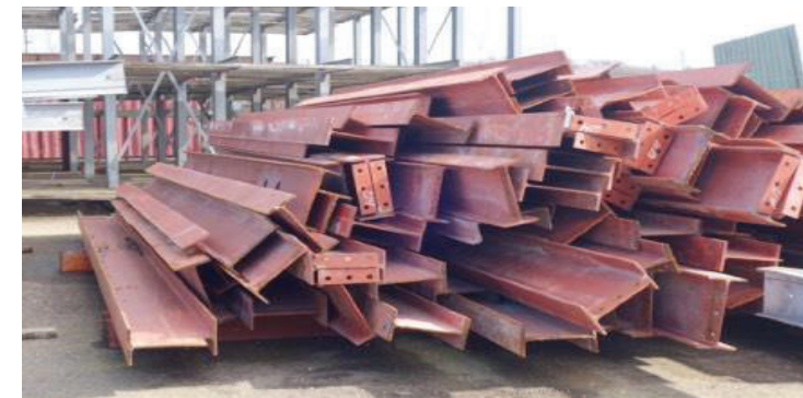
Bedzed Project (2002), Hackbridge (UK). Reuse of 95 tonnes of steel
